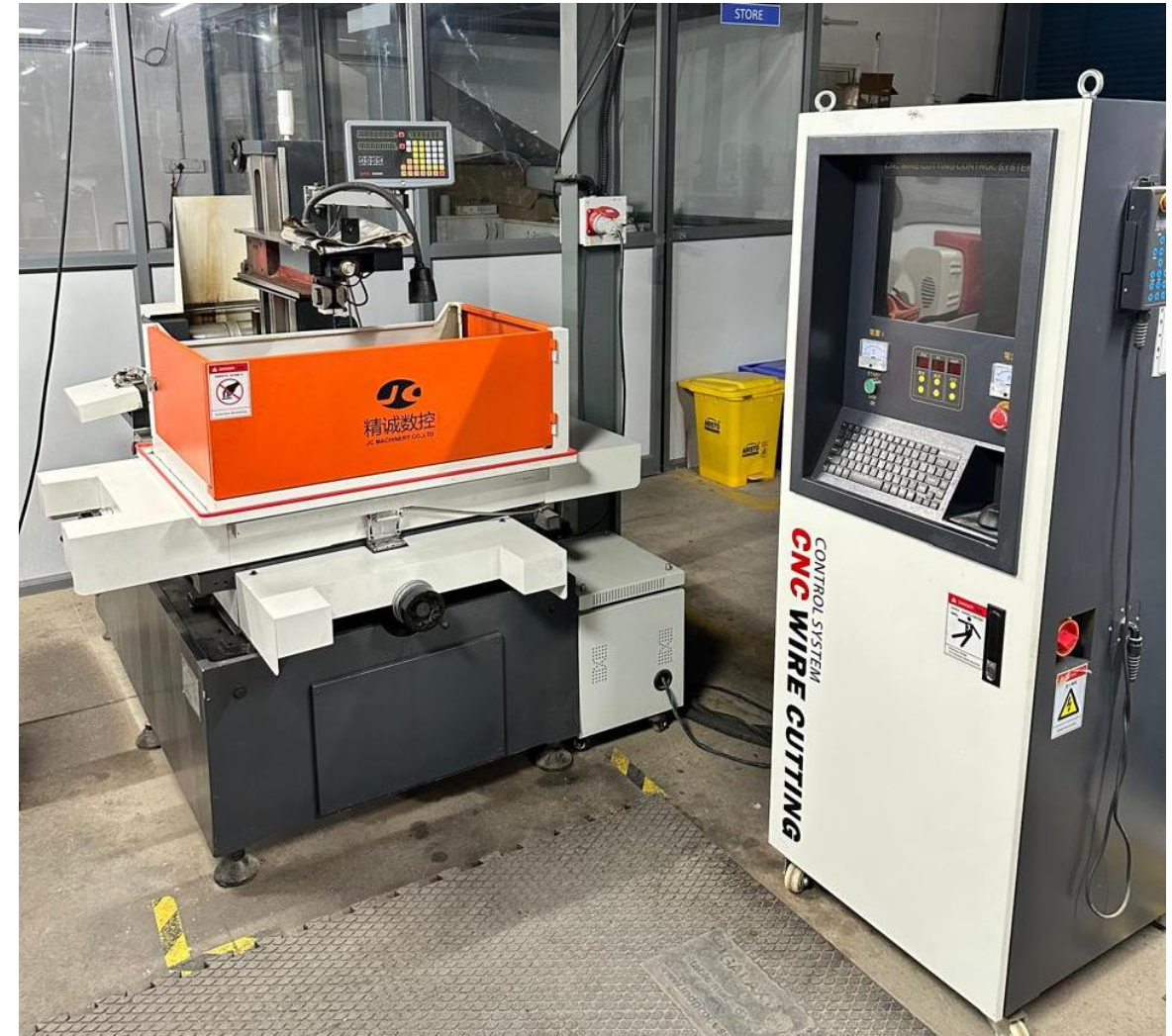
SEMI PRECISION WIRECUT 400mm X 300mm X 300mm TAIWANESE COMPANY
