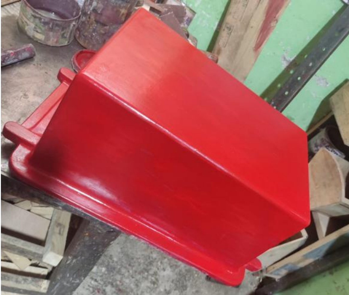
Wooden pattern used for Al casting
