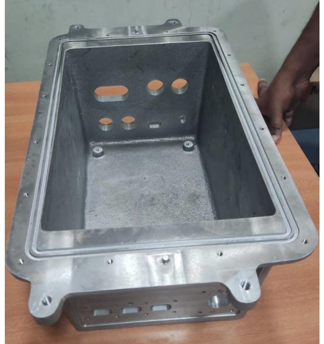
PDU Boxes after Machining
