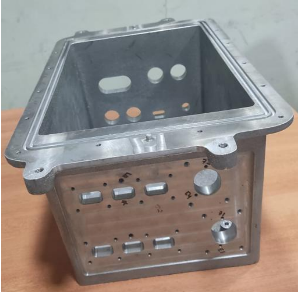
PDU Boxes after Machining
